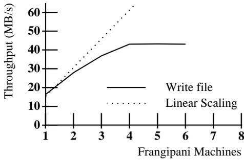
**Figure 7: Frangipani Scaling on Write.** Each Frangipani server writes a large private file. The dotted line shows the linear speedup curve for comparison. Performance tapers off early because the ATM links to the Petal servers become saturated.
