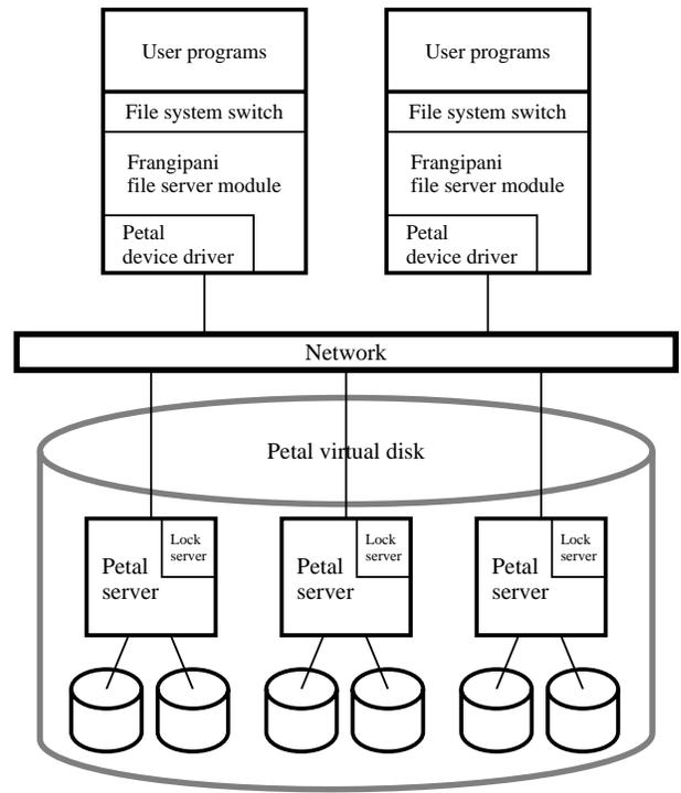
**Figure 2: Frangipani structure.** In one typical Frangipani configuration, some machines run user programs and the Frangipani file server module; others run Petal and the distributed lock service. In other configurations, the same machines may play both roles.
