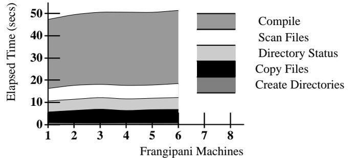
**Figure 5: Frangipani Scaling on Modified Andrew Benchmark.** Several Frangipani servers simultaneously run the Modified Andrew Benchmark on independent data sets. The y-axis gives the average elapsed time taken by one Frangipani machine to complete the benchmark.
