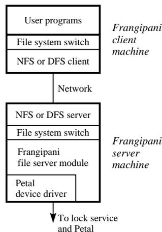
**Figure 3: Client/server configuration.** A Frangipani server can provide file access not only for the local machine, but also for remote client machines that connect via standard network file system protocols.
