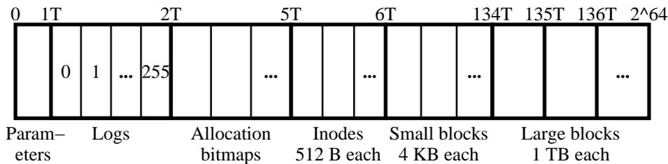
**Figure 4: Disk layout.** Frangipani takes advantage of Petal’s large, sparse disk address space to simplify its data structures. Each server has its own log and its own blocks of allocation bitmap space.
