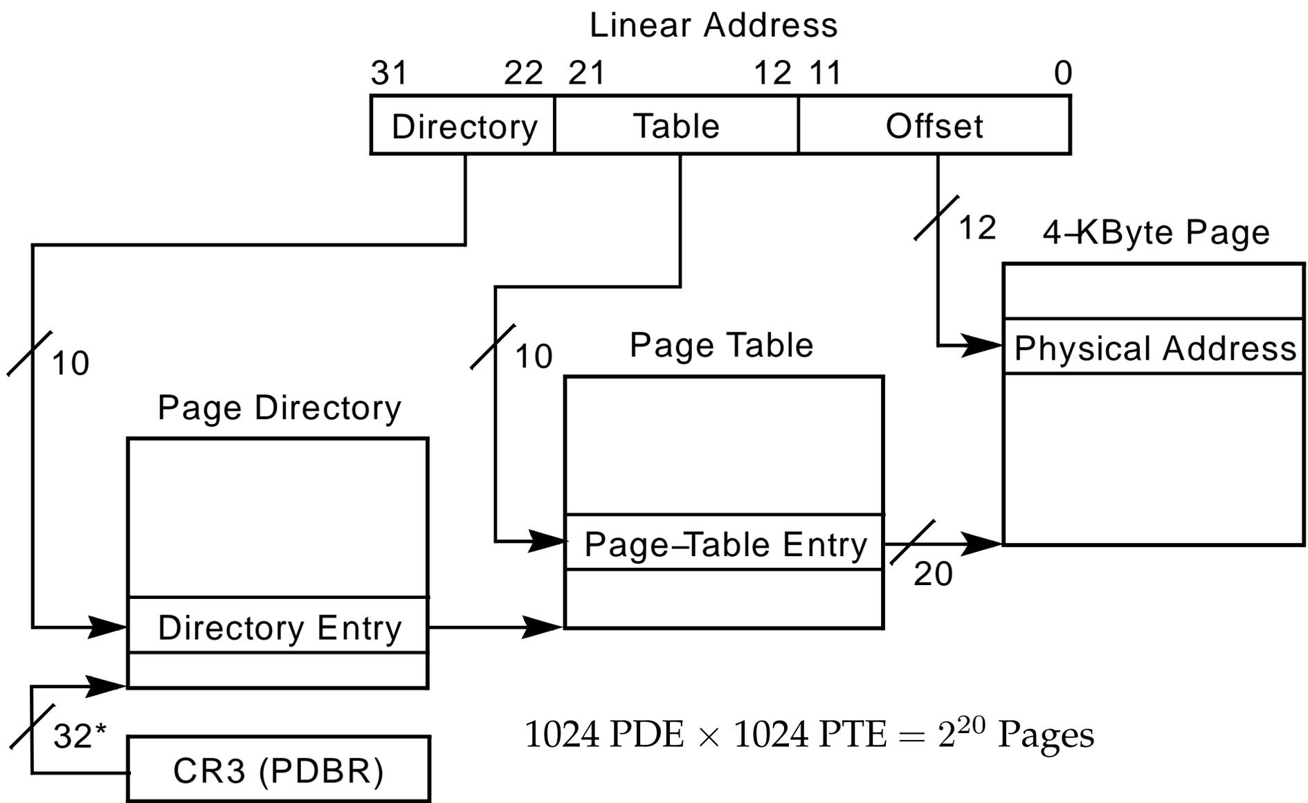
\*32 bits aligned onto a 4-KByte boundary
