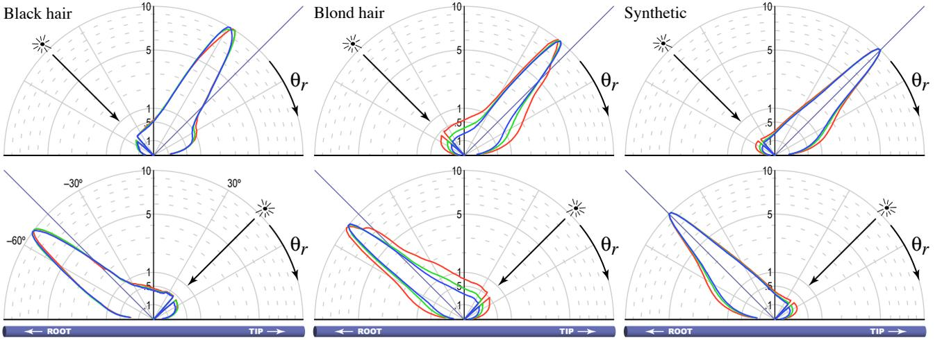
Figure 4: Measurements of scattering in the incidence plane: scattering as a function of scattering angle with illumination at  $45^\circ$  from the tip and root ends. Black and blond hair are shown, along with a synthetic fiber from a wig.
