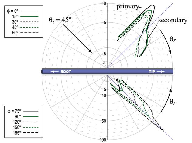
Figure 8: A measurement of one hemisphere of the scattered distribution for a fixed incidence direction with angle of incidence  $45^\circ$ . The primary highlight, the secondary highlight, and the transmitted component are all visible.
