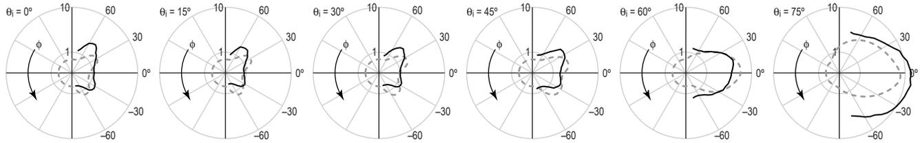
Figure 6: A measurement showing the evolution of glints with incidence angle on a more nearly circular hair. For each  $\theta$  the source is fixed while the camera sweeps along the specular cone. A qualitative match to our shading model is plotted with dashed curves.
