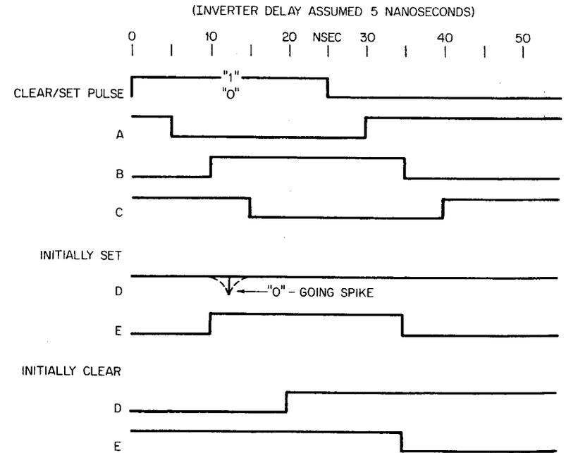
FIGURE 19 Flip-flop logical representation and timing chart.
