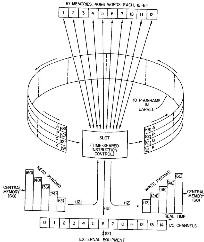
FIGURE 83 Peripheral processors.
