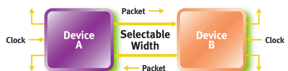
Figure 8. A PCI Express™ link uses transmit and receive signal pairs.
